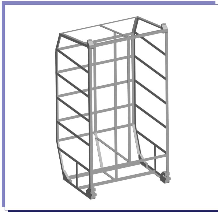
Figure 7-25: International Standard Payload Rack (ISPR): 6-post configuration
