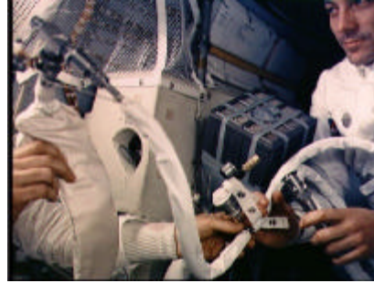
Figure 11: Swigert with temporary hose connections and apparatus required when the crew moved from the CM to the LM (NASA AS13-62-9004).
