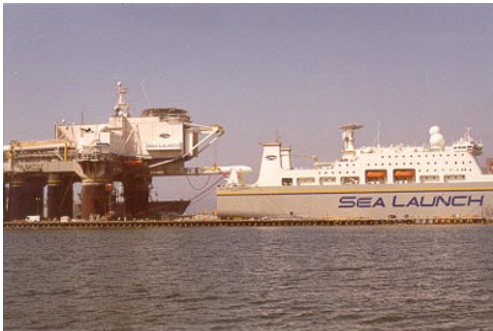
Figure 9-8. Launch Vehicle Transfer from Assembly and Command Ship to Launch Platform at Home Port
