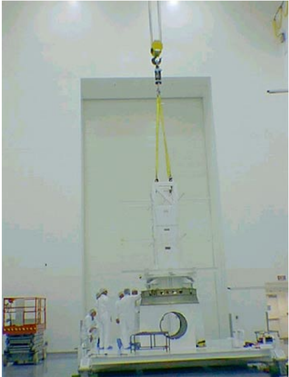
Figure 8-5. Fit Check on Adapter Support Stand
