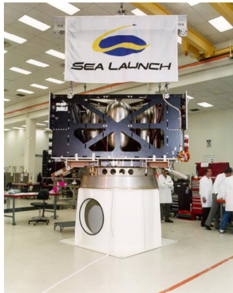
Figure 6-7. Electrical and Mechanical Mates
