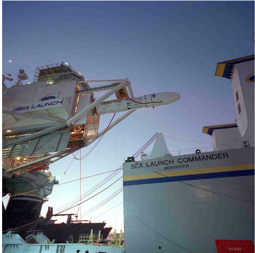
Figure 8-18. Lifting of Integrated Launch Vehicle
