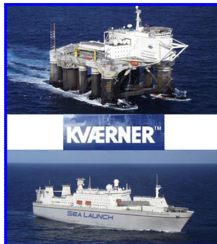
Figure 1-6. Launch Platform and Assembly and Command Ship
