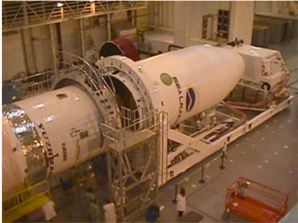
Figure 8-16. Payload Unit Mating to the Zenit-3SL
